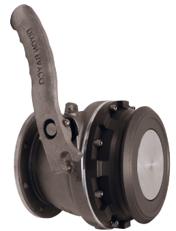
API adapter with fixed handle (poppet can open with API coupler engagement or by using the handle) 5204NG
