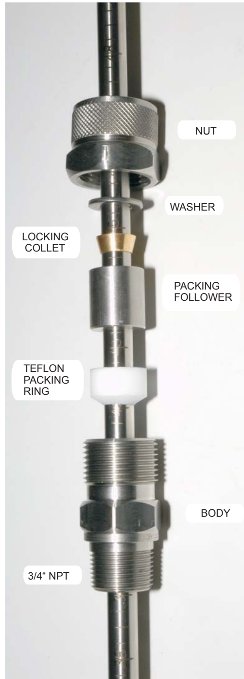
EXPLODED VIEW, 3/4" 300 LB SLIDING FITTING
