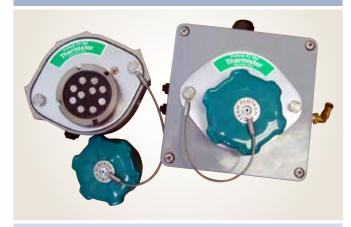
Sockets allow for the transfer of the electronic signal from the terminal control monitor to the tanker. Sockets will vary depending upon terminal equipment.
